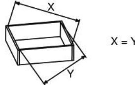
**Attention! The bottom of the drawer should be nailed after setting up the diagonal between the elements (see drawing).**
