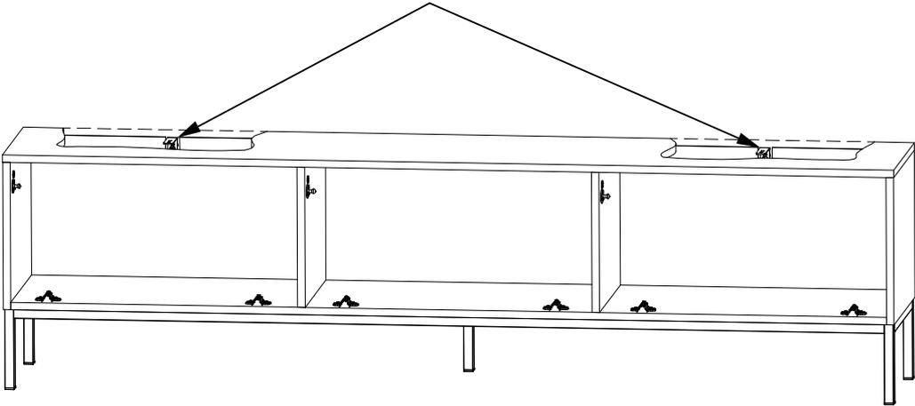
1. KR connector is placed on the top rail of the cabinet.
